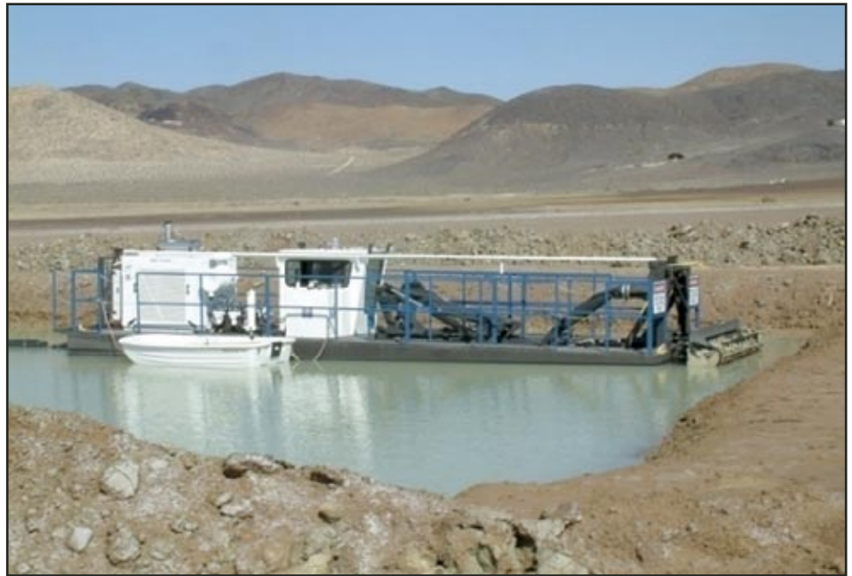
Columbus Mine Dredge (pictured above) allows mined material to be handled as a slurry throughout the production process – a significantly low cost method to prepare mined materials for extraction of precious metals in Ireland's pilot production mill facility (pictured below).
